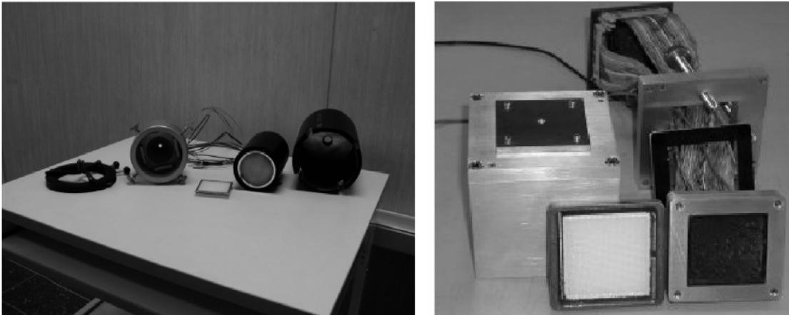
Figure 25: Two detector setups using different photodetectors. At left: NaI(Tl) pixellated array (1.8 x 1.8 x 6 mm ) coupled with R2486 Hamamatsu PSPMT using pinhole collimator. At right: The same system but using H8500 PSPMT as photodetector.
