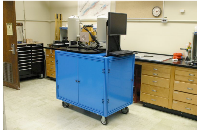
Figure 43: The first generation Si+Ge Compton imaging system (CCI-1), which mounted on a cart.
