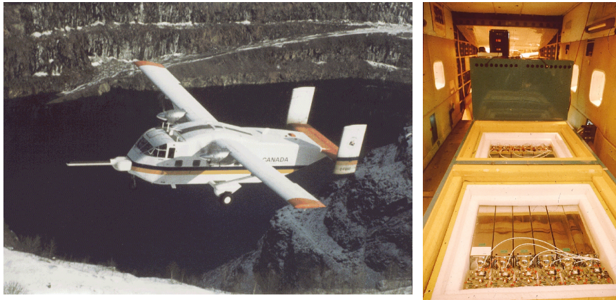
Figure 8: The Canadian Skyvan of the Canadian Geological Surveillance Canada (left) with 14 large volume NaI detectors with a total volume of 50 l on board (right).
