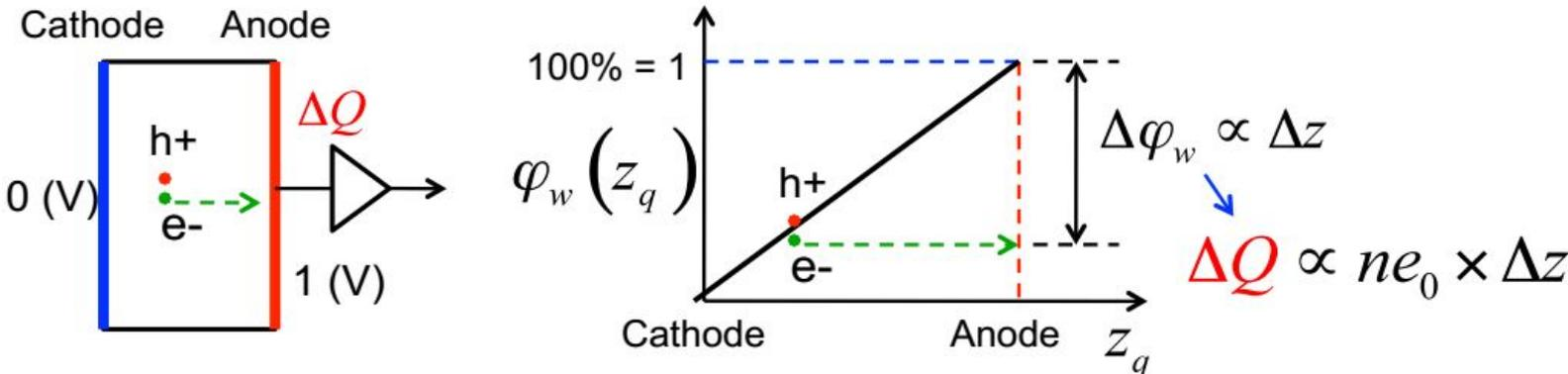
Single-polarity charge sensing using **pixelated** anode electrodes
