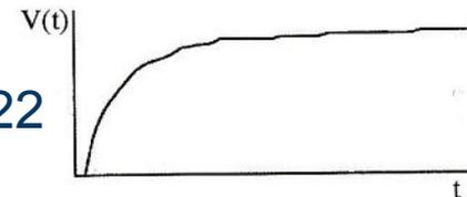
Leading edge of voltage pulse across anode circuit with long time constant
